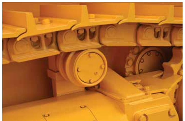
Working loads from the blade and rear mounted attachments are evenly distributed through the frame and undercarriage.
